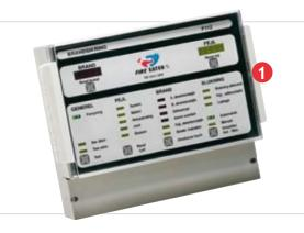
The control panel is self-monitoring, which means that it continuously tests whether all circuits are intact and ready for use. If the control panel encounters a fault which may cause the system to be un-operational, it will indicate system fault.
